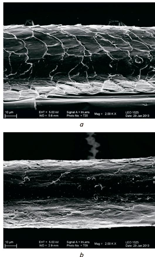
Fig. 1. Microphotographs of the surface of coarse wool fiber: *a* – untreated fiber; *b* – EDNBC-modified fiber
