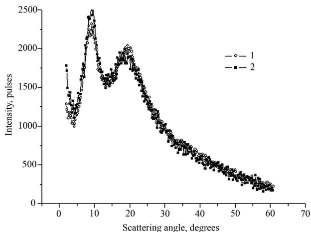
Fig. 2. Wide-angle scattering diffractogram of the coarse wool samples: 1 – untreated fiber; 2 – EDNBC-modified fiber
