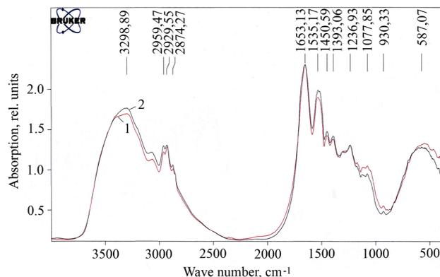
Fig. 3. IR-spectra of coarse wool fiber: 1 – untreated fiber; 2 – EDNBC-modified fiber
