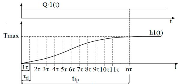
Fig. 3. Splitting the time of transition process into  $n$  equal intervals over time:  $T_{max}$  is the maximum temperature at studied point,  $t_{tp}$  is the time of transitional processes,  $\tau_d$  is the time of transport delay,  $Q$  is the amplitude of heat flow
