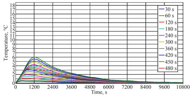
Fig. 9. Influence of durations of a heater that is turned on on indoor temperature
