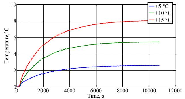
Fig. 6. Reaction of object of control to temperature change by +5 °C, +10 °C and +15 °C
