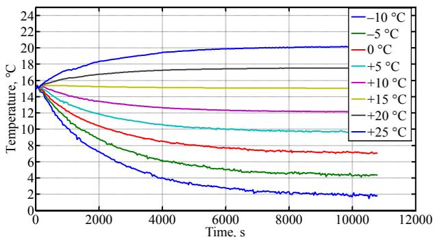
Fig. 5. Influence of outdoor temperature on indoor temperature at initial temperature +15 °C
