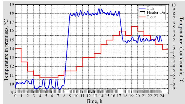
Fig. 10. Results of the experiment applying a method of the PWM predictive control: T in – temperature at the set point inside premises, Heater On – operating time of the heater, T out – outdoor air temperature
