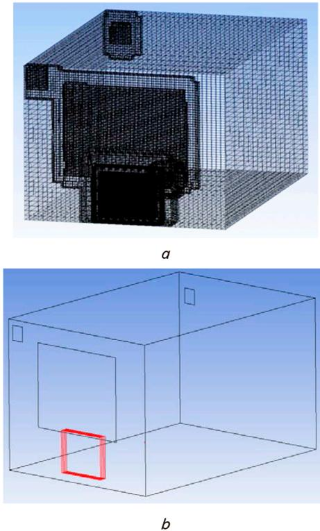
Fig. 2. 3-dimensional model of a building's block of the examined object: a - general view, b - splitting into finite elements
