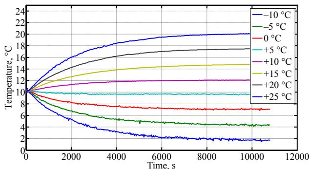
Fig. 4. Influence of outdoor temperature on temperature in premises at initial temperature +10 °C
