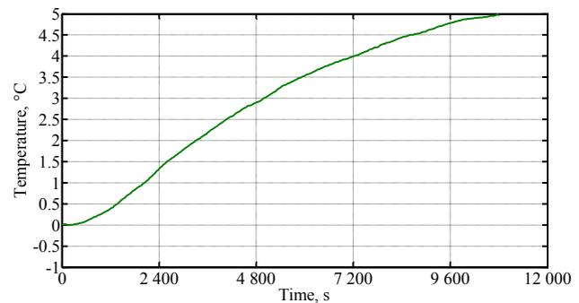
Fig. 7. Transitional characteristic of ventilation at air temperature equal to 18 °C
