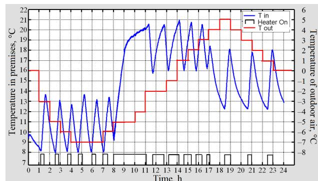
Fig. 12. Results of experiment using a two-position controller with the magnitude of hysteresis equal to 2 °C: T in – temperature at a given point inside premises, Heater On – operating time of the heater, T out – outdoor air temperature
