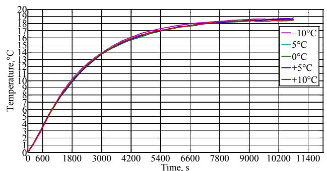
Fig. 8. Transitional characteristic of the control object when the heater is on
