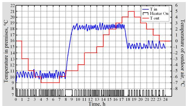
Fig. 11. Results of experiment using a two-position controller without hysteresis: T in – temperature at a given point inside premises, Heater On – operating time of the heater, T out – outdoor air temperature
