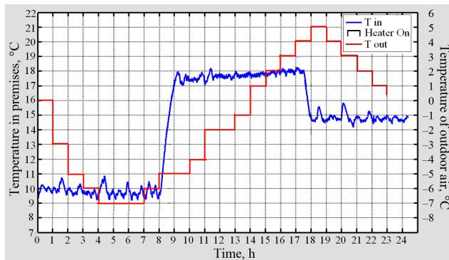
Fig. 13. Results of experiment using a PID-controller: T in – temperature at a given point inside premises, Heater On – operating time of the heater, T out – outdoor air temperature
