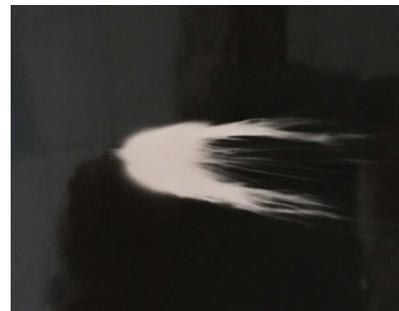
Fig. 11. Arc discharge and particle flows of the sprayed flux-cored electrodes with pressure drop in the center
