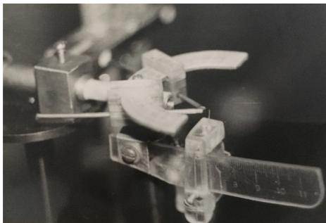
Fig. 5. Scheme and appearance of the working part of the installation for determining  $P_{\Sigma}$
