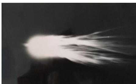
Fig. 10. Arc discharge and particle flows of the sprayed flux-cored electrodes
