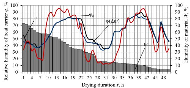
Fig. 6. Kinetic parameters of the moisture release processes in the solar dryer over the period of 10–12.08. 2017
