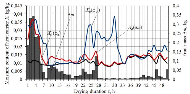
Fig. 7. Dynamics of the mass transfer processes in the solar dryer over the period of 10–12.08.2017
