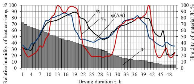
Fig. 3. Kinetic parameters of the processes of moisture release in the solar dryer over the period of 15–17.07.2017:  $\phi_i$ ,  $\phi_o$  are, respectively, the relative humidity of the incoming and outgoing flows of heat carrier, %;  $W$  is the humidity of the material being dried, %;  $\phi(\Delta m)$  is the simulated time dependence of the humidity of outgoing flow of heat carrier, %
