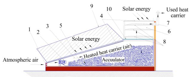
Fig. 1. Structural-technological circuit of the solar dryer with a heat accumulator and a flat mirror concentrator: 1 – inlet channel; 2 – fan; 3 – air duct; 4 – air collector; 5 – heat-accumulating material (gravel-based); 6 – drying chamber; 7 – return channel; 8 – sieves; 9 – flat mirror concentrator; 10 – valve
