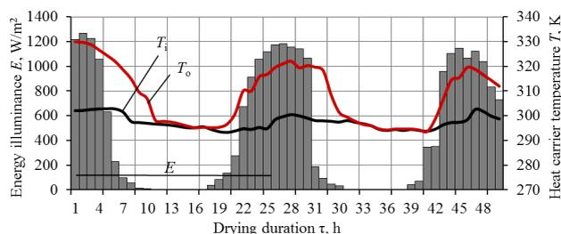
Fig. 2. Energy parameters of the solar dryer operation over the period of 15–17.07.2017:  $T_i$ ,  $T_o$  are, respectively, the temperature of the incoming and outgoing heat carrier, K;  $E$  is the energy illuminance, W/m<sup>2</sup>
