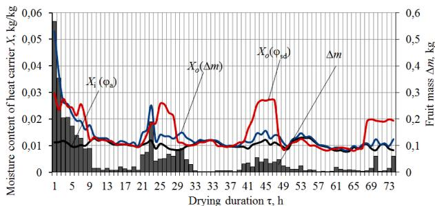
Fig. 8. Dynamics of the mass transfer processes in the solar dryer over the period of 28–31.07.2017
