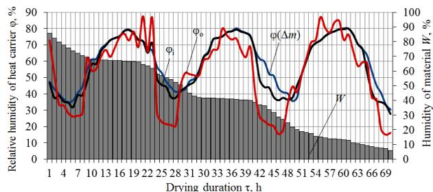
Fig. 9. Kinetic parameters of the moisture release processes in the solar dryer over the period of 28–31.07.2017
