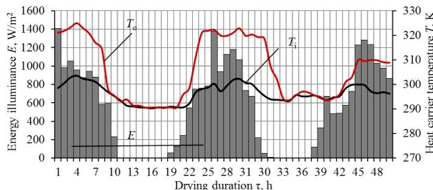
Fig. 5. Energy parameters of the solar dryer operation over the period of 10–12.08.2017
