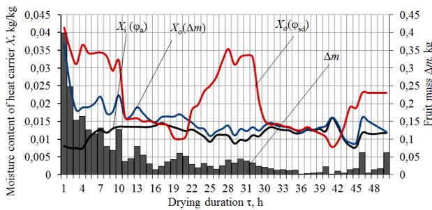
Fig. 4. Dynamics of processes of mass transfer in the solar dryer over the period of 15–17.07.2017:  $X_i(\varphi_a)$ ,  $X_o(\varphi_{sd})$  are, respectively, the moisture content of the incoming and outgoing flows of heat carrier, kg/kg;  $\Delta m$  is the hourly change in the mass of material being dried, kg;  $X_o(\Delta m)$  is the simulated time dependence of moisture content in the outgoing flow of heat carrier, kg/kg
