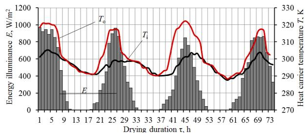
Fig. 10. Energy parameters of the solar dryer operation over the period of 28–31.07.2017 without a dryer
