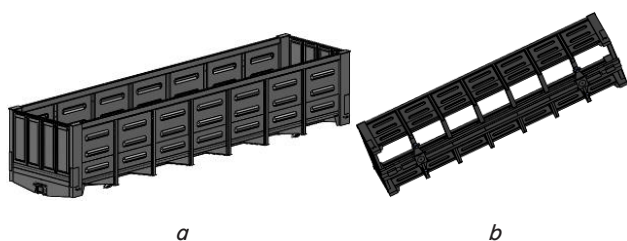
Fig. 4. Spatial model of an open top wagon with the wear characteristic of 1.5 terms of operation: a – side view; b – bottom view
