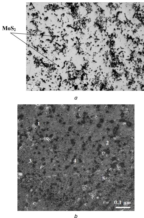
Fig. 1. Structure of AM4.5Kd+10 % MoS<sub>2</sub>: *a* – distribution of MoS<sub>2</sub> indicated by arrows, there is a section not etched; *b* – is an image of intermetallic (1 – CuAl<sub>2</sub>, 2 – MnAl<sub>6</sub>, 3 – NiAl<sub>3</sub>, 4 – TiAl<sub>3</sub>, 5 – Al<sub>2</sub>CuMn), there is a section etched (NaOH). We obtained the image from a metallographic microscope
