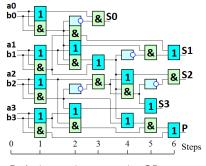
Fig. 7. 4-bit acyclic adder with OR elements in the last digit
