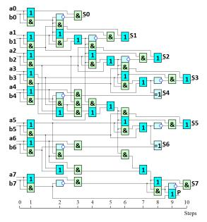
Fig. 14. The 8-bit acyclic PAA with the circuit depth of 10 standard 2-input elements
