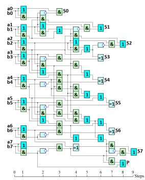
Fig. 11. Acyclic 8-bit PAA with circuit depth of 9 standard 2-input elements
