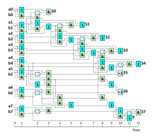
Fig. 19. The 8-bit acyclic PAA with the circuit depth of 12 standard 2-input elements
