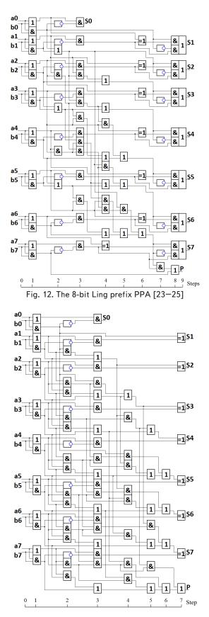
Fig. 13. The 8-bit Kogge-Stone prefix PPA [3, 8] and the 8-bit Knowles PPA [26, 27]
