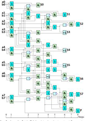
Fig. 9. Acyclic 8-bit PAA with circuit depth of 8 standard 2-input elements
