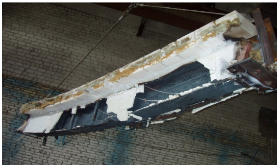
Fig. 6. Physical appearance of a loaded beam with the passive fire-protective material after the test
