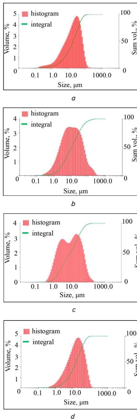
Fig. 3. The particle size distribution by volume: *a* – CEM I 42.5 R; *b* – GBFS-3; *c* – SZ; *d* – SFA
