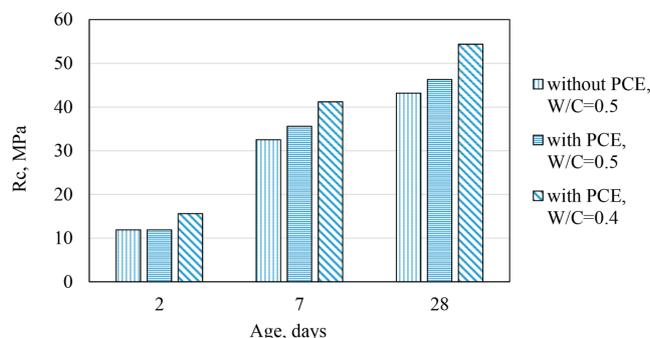
Fig. 8. Influence of PCE superplasticizer on compressive strength of low-emission ternary pozzolanic cement
