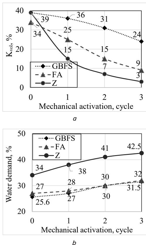
Fig. 2. Effect of mechanical activation on physical properties of SCMs: *a* – bleeding ( $K_{vol}$ ); *b* – water demand (*WD*)
