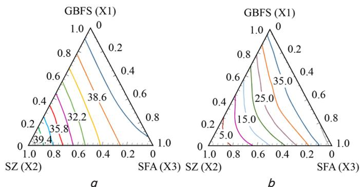
Fig. 6. Isolines of influence of composition of SCMs based on GBFS, super-zeolite and fly ash on: a – bleeding; b – water demand
