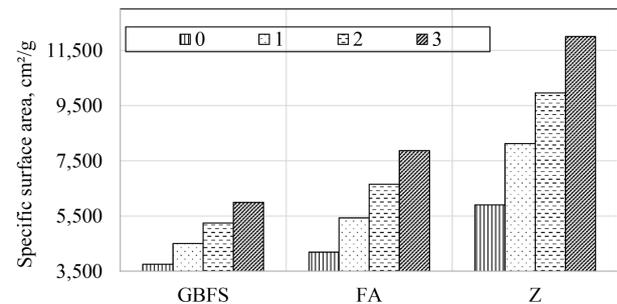
Fig. 1. Dispersion of SCMs after mechanical activation
