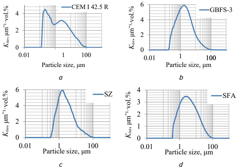
Fig. 4. The particle size distribution by surface area for: a – CEM I 42.5 R; b – GBFS-3; c – SZ; d – SFA
