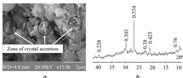
Fig. 7. Stone on the basis of the GBFS-SZ-SFA system after 180 days of hardening: a – microstructure; b – phase composition
