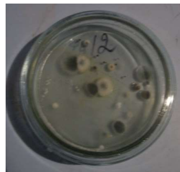
Fig. 9. Colonies of Penicillium and Fusarium fungi in Chapek medium, extracted from a concrete without admixtures
