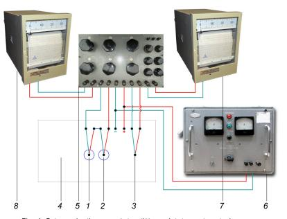
Fig. 1. Schematic diagram of the differential thermal analysis setup: 1 – sample with a thermocouple; 2 – standard with a thermocouple; 3 – thermocouple for recording the temperature in the chamber of microrefrigerators; 4 – micro-refrigerators TLM-2 (USSR); 5 – two-coordinate potentiometer R-307 (Russia, Krasnodar); 6 – power supply unit for microrefrigerators VSP-33 (USSR, Lviv); 7, 8 – paper recorder (USSR, Lviv)
