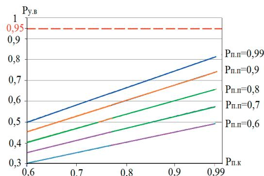
Fig. 5. Dependence of GSC effectiveness ( $P_{S,f}$ ) on  $P_{c,c}$  and  $P_{c,r}$  during placement of one  $SS$  in far or close control zones
