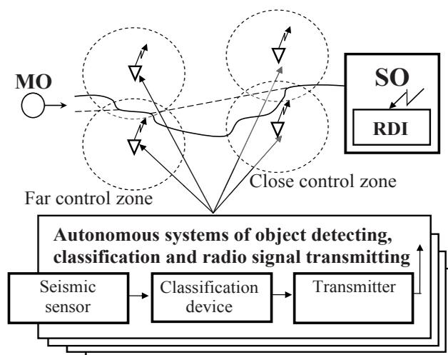
Fig. 1. Layout of placement of GSC systems
