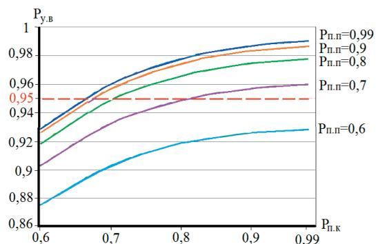
Fig. 2. Dependence of GSC effectiveness ( $P_{S,f}$ ) on  $P_{c,c}$  and  $P_{c,r}$  during placement of four  $SS_S$  in pairs in far and close control zones
