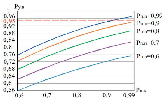
Fig. 4. Dependence of GSC effectiveness ( $P_{S,f}$ ) on  $P_{c,c}$  and  $P_{c,r}$  during placement of two  $SS_S$  serially in far and close control zones
