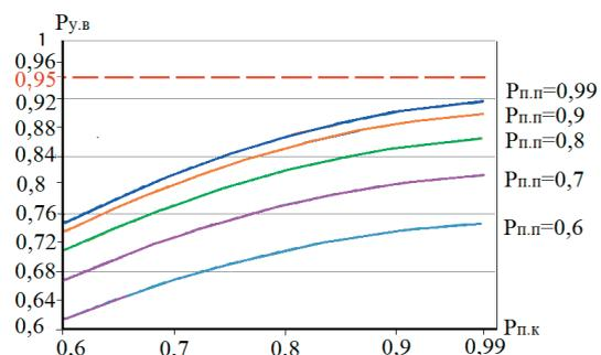
Fig. 3. Dependence of GSC effectiveness ( $P_{S,f}$ ) on  $P_{c,c}$  and  $P_{c,r}$  during placement of two  $SS_S$  on the border in far and close control zones
