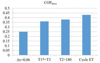
Fig. 8. The coefficient of performance of the theoretical cycle  ${\rm COP}_{\it theor}$  with extended degazation zone
