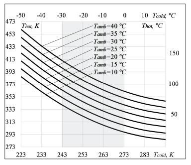
Fig. 2. Theoretical minimum temperature  $T_{\rm hot}$  depending on temperatures  $T_{\rm cold}$  and  $T_{\rm amb}$
