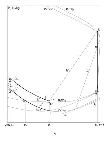
Fig. 7. The scheme and cycle of a thermochemical compressor with a reverse supply of solution to the generator and absorber: a – technological scheme; b – cycle in the h-x diagram
