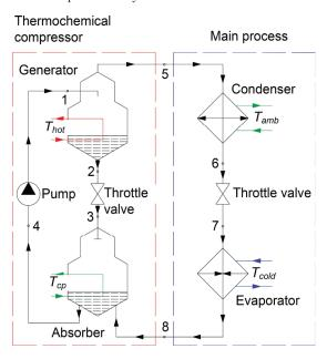
Fig. 1. Simple absorption thermotransformer
