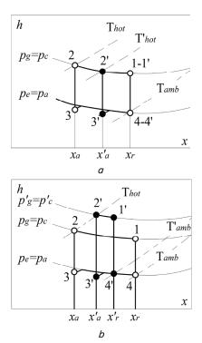
Fig. 3. Dynamics in the narrowing of the degazation zone in a thermochemical compressor: a — lowering the temperature of the heating source  $\left(T_{hot}^{!} < T_{hot}\right)$ ; b — increasing ambient temperature  $\left(T_{amb}^{!} > T_{amb}\right)$
