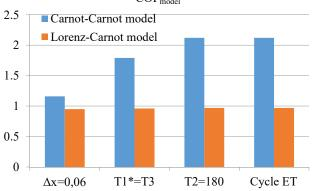
Fig. 9. The coefficient of performance for the cycle models with extended degazation zone
