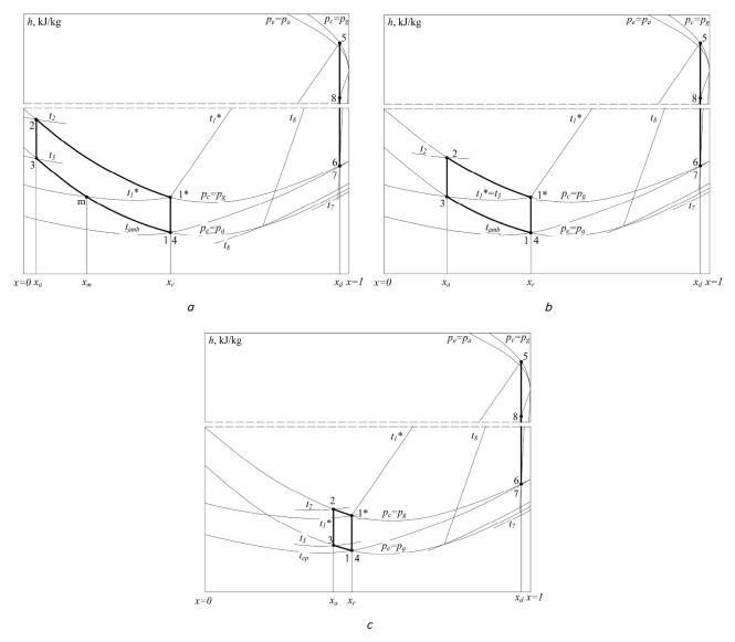
Fig. 6. Cycles in the hx enthalpy–concentration diagram: a – cycle  $\Delta x$ =0.06; b – cycle  $T_1*=T_3$ ; c – cycle  $T_1*< T_3$
