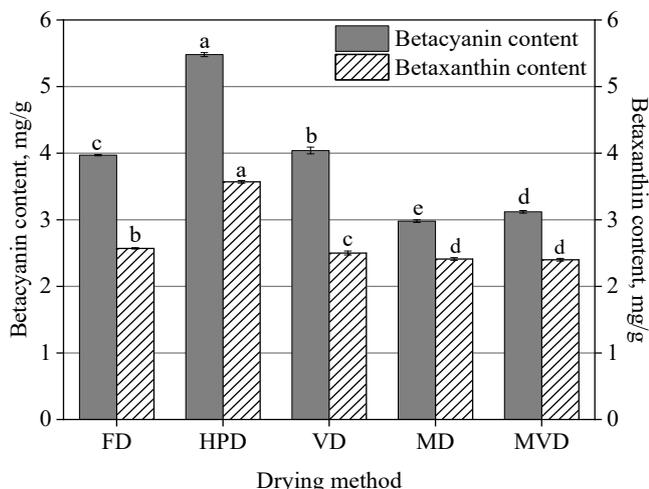
Fig. 4. Betalain content of dried beetroots prepared by different drying methods, different letters indicate significant differences at  $p < 0.05$  according to Duncan's multiple test
