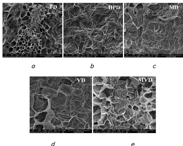
Fig. 3. Microstructure (500× magnification) of dried beetroots prepared by different drying methods: a – FD; b – HPD; c – MD; d – VD; e – MVD
