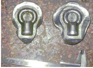
Fig. 9. Comparison of forgings with flash, the left one was profiled with buckling and the right one was manufactured according to the conventional technology
