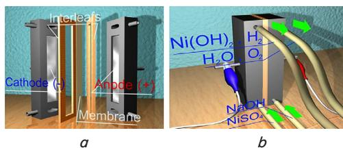
Fig. 1. Slit diaphragm electrolyzer: *a* – components, *b* – assembled
