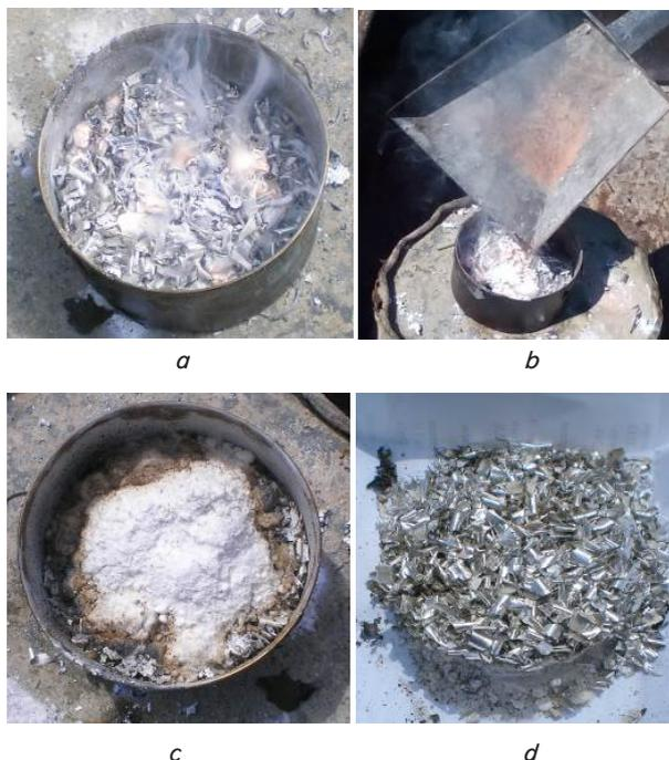
Fig. 4. Results of tests of extinguishing magnesium flame with a model sample of dry mixtures coating with the addition of minerals: a – magnesium ignition, b – extinguishing of flame, c – formation of combustible substance of the insulation layer on a surface, d – results of extinguishing
