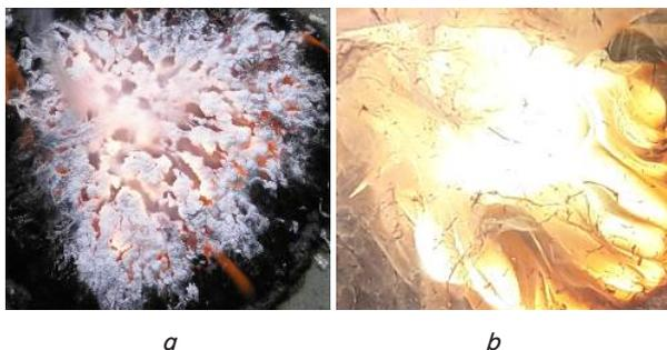
Fig. 3. Results of extinguishing magnesium flame with wet sand: a – combustion of magnesium; b – throwing of a wet sand in a magnesium flame
