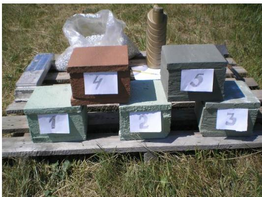
Fig. 1. Model samples of containers for the storage of weapons and ammunition that were treated with an organic coating with an addition of: 1 – aluminosilicate microspheres; 2 – perlite; 3 – basalt scales; 4 – metallurgical sludge; 5 – ashes
