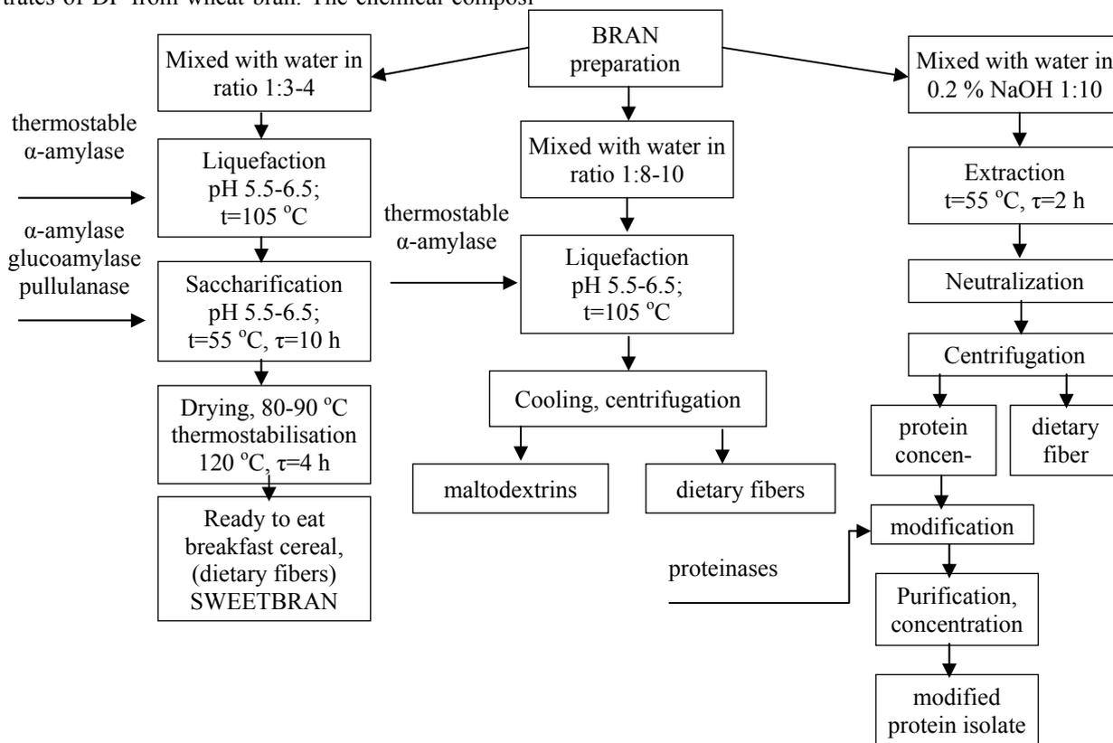
Fig. 3. Processes for making DF, modified protein isolate and maltodextrins
