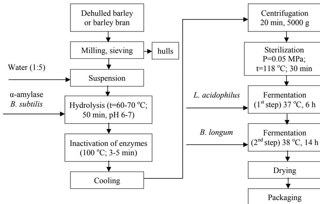
**Fig. 4. Process for making a functional cereal bioproduct from barely**
