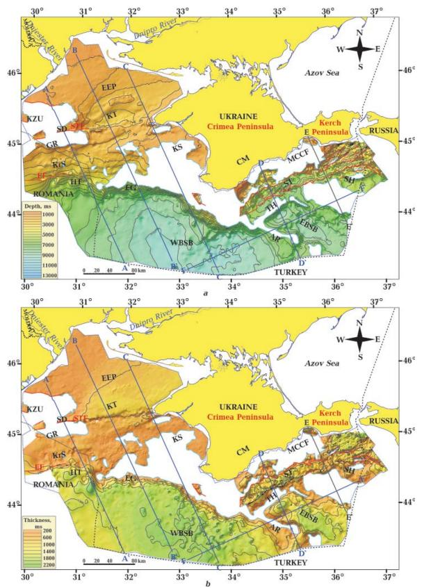
Fig. 15. TWT structural map at the base of the Oligocene (lower part of Maykopian) sediments (*a*) and TWT thickness map of the Oligocene sequence (*b*) for the study area. See Fig. 2 for abbreviations of tectonic units and Fig. 9 for other explanations and abbreviations.
