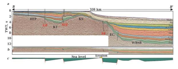
Fig. 4. Interpreted seismic reflection profile B—B'. See Fig. 3 for explanation; see also Fig. 2 for abbreviations of regional tectonic units and Fig. 3 for abbreviations of sedimentary sequences. Abbreviations of fault names (in red): GF — Golitsin Fault; EF — Euxinian Fault; STF — Sulina—Tarkhankut Fault.
