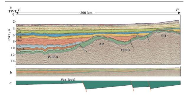
Fig. 8. Interpreted seismic reflection profile F—F'. See Fig. 3 for explanation; see also Figs. 2, 3 for abbreviations of regional tectonic units and sedimentary sequences.
