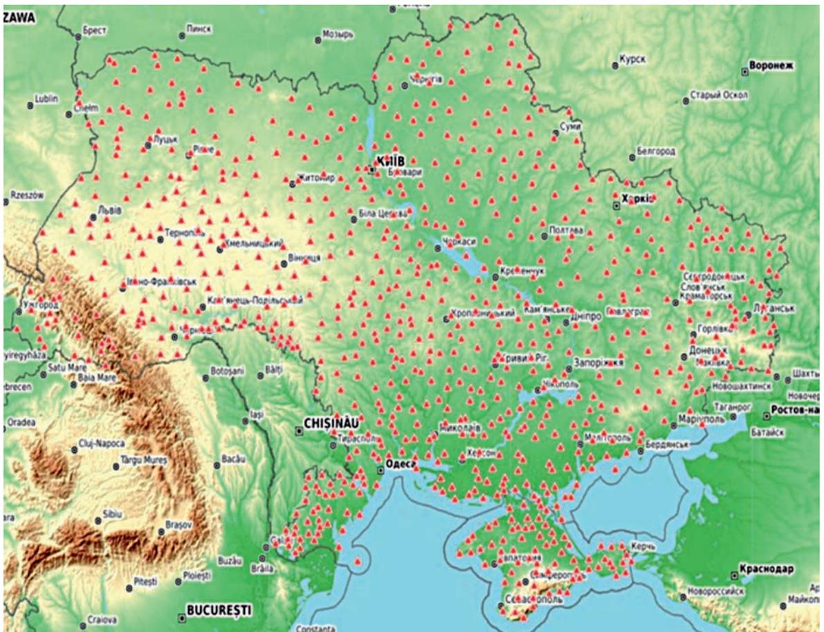
Fig. 6. Map-scheme of the geodetic (planned) network of the 1st class of Ukraine.
