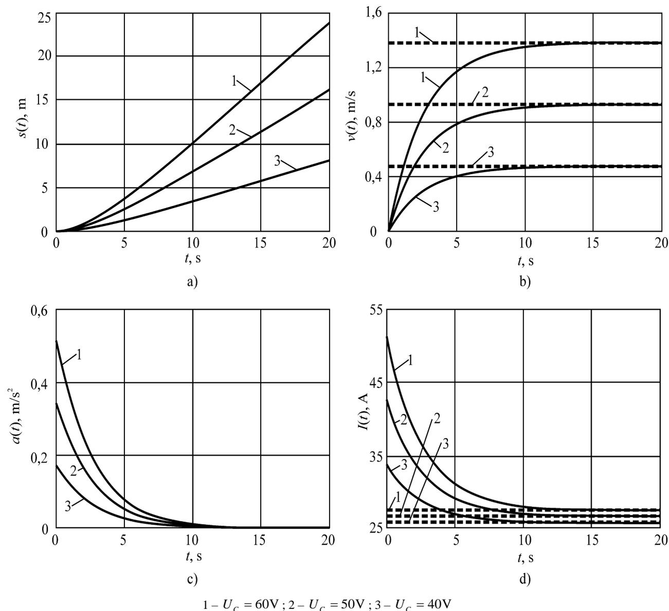
**Fig. 3.** Results of computer simulations (solid) of the translational coordinate (a), the velocity (b), the acceleration (c) and for the electric current (d) in the drive electric motors for the robotic wheeled platform, as well as the theoretically predicted results (dash) for the steady state
