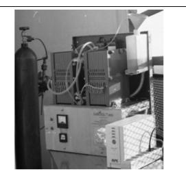
Fig. 5. Hydrogen/air fuel cell with power 0.4 kW
