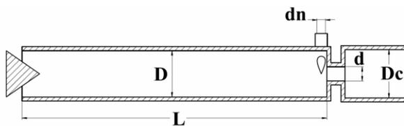
Fig. 1. Schematic view of the vortex tube geometry
