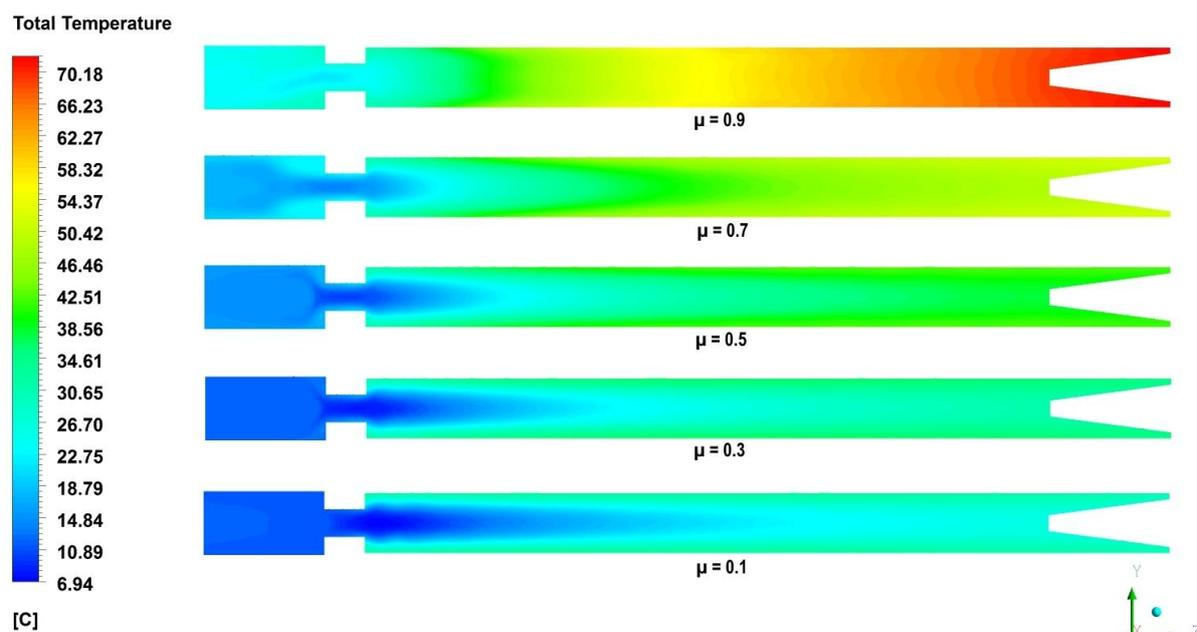
Fig. 6. Contours of total temperature in YZ plane
