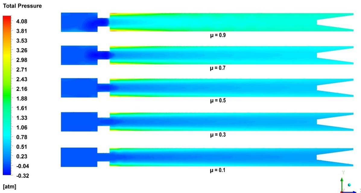
Fig. 5. Contours of total pressure in YZ plane
