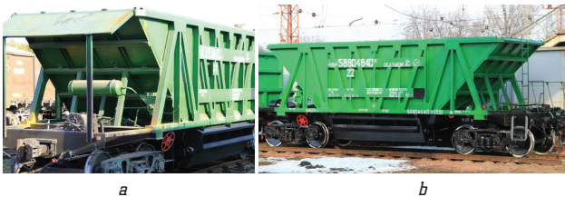
Fig. 1. Hopper wagon for transportation of pellets: a – end view; b – side view
