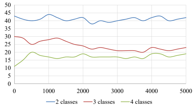
Fig. 2. Dependency of the accuracy of data classification depending on the amount of data and the number of categories using the Bloom filter
