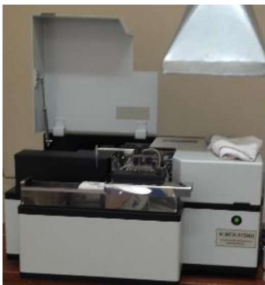
Figure 5. Atomic adsorption spectrometer MGA-915MD
