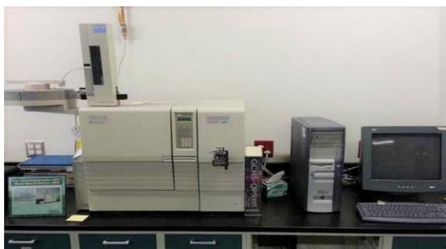
Fig. 2. Gas chromatograph GC-17A “Shimadzu” with the software “GC solution”, (Japan)
