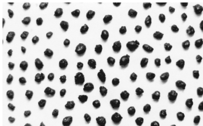
Fig. 9. Coal-oil fuel aggregates-granules obtained based on Donetsk coal of 0–1 mm. The mean dimensionality of aggregates is 2–3 mm
