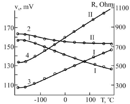
Fig. 7. Temperature dependences of Hall voltage (1, 2) and resistance (3, 4) for both I and II types of hallotrons
