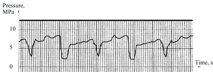
Fig. 4. Experimental curves of oil pressure variation in the pressure pipeline
