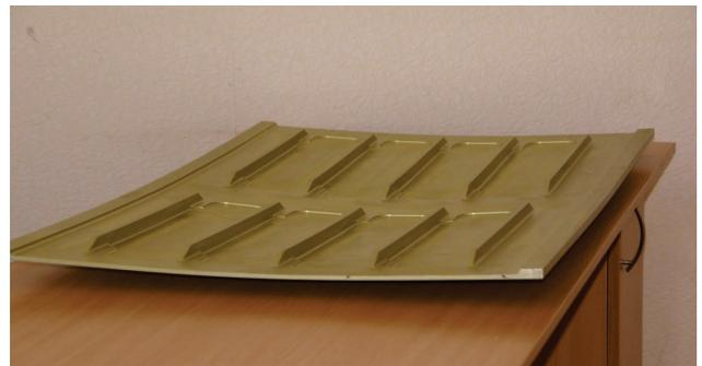
Fig. 7. A double-curvature panel with a complex internal engraving formed by the method of local bending with stretching
