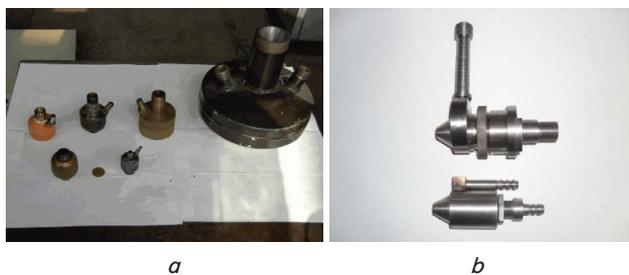
Fig. 7. Hydrovortex nozzles: *a* – for emulsion fuels; *b* – for suspension fuels
