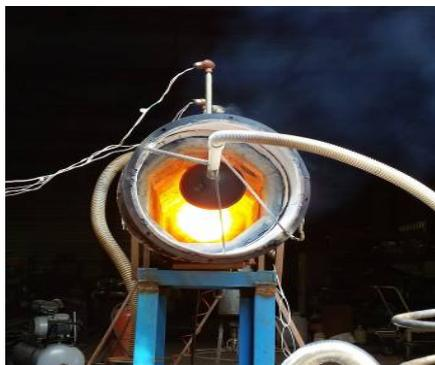
Fig. 11. The process of combustion of a composite fuel with the addition of spent FF
