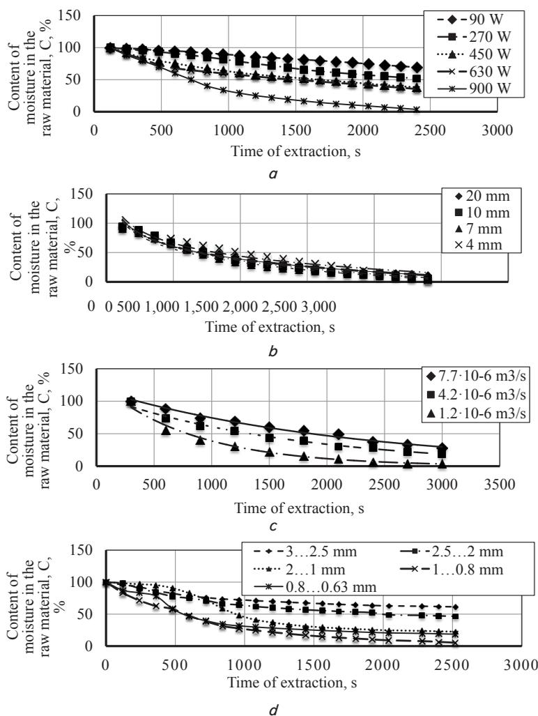
Fig. 7. The kinetics of mass transfer of water-soluble substances in the MW field: a – the influence of the MW field force; b – the thickness of the layer; c – the consumption of the extractant; and d – the size of the fractions
