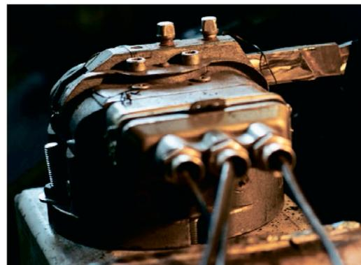
Fig. 3. Measuring head UDM-100 with a cutter
