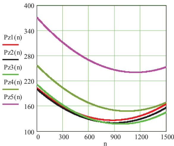
Fig. 4. Charts of functions  $P_z(n)$  investigated for the extremum at spindle rotation frequency  $n$
