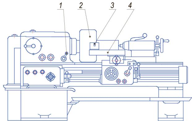
Fig. 2. Schematic of the experimental installation for shredding tires by cutting: 1 – lathe-screw machine 16K20; 2 – pneumatic tire; 3 – measuring head UDM-100 with a cutter; 4 – transitional console
