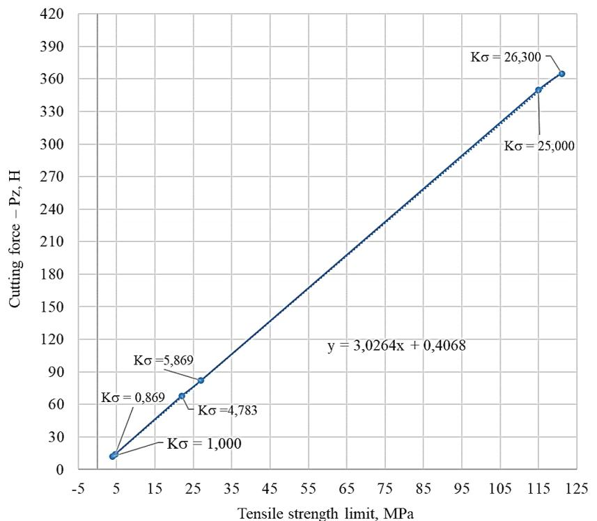
**Fig. 7.** Chart of dependences of cutting force on tensile strength limit of materials of different tires
