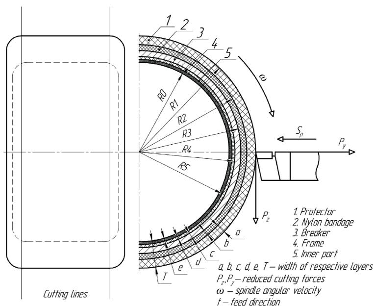
Fig. 1. Location diagram of the reduced cutting forces  $P_z$  and  $P_y$  along coordinate axes
