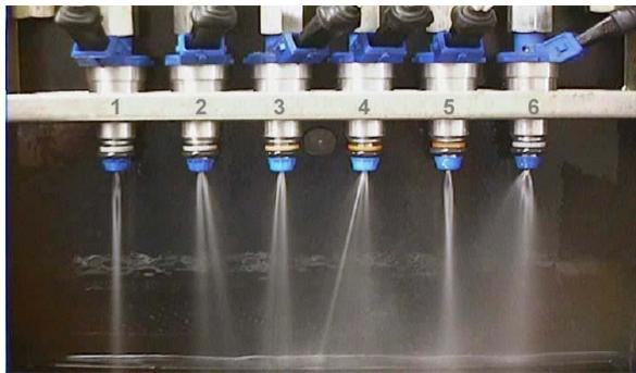
Fig. 1. Visual assessment of the degree of fuel atomization by injectors
