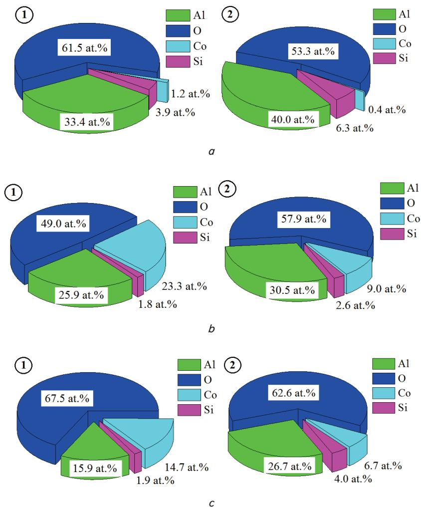
Fig. 5. Chemical composition of plots 1 and 2 (Fig. 4) on oxide coatings obtained in electrolytes of following composition, mol/dm<sup>3</sup>:
