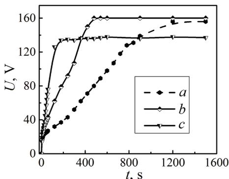
Fig. 1. Chronograms of forming voltage during PEO of AK12M2MgN in electrolytes of the following composition, mol/dm<sup>3</sup>:
