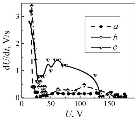
Fig. 2. Rate of voltage change during PEO of AK12M2MgN in electrolytes with different composition, mol/dm<sup>3</sup>:
