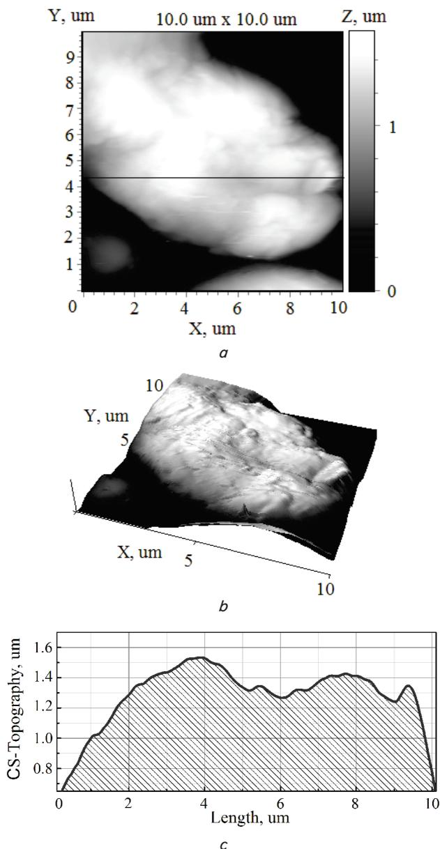
Fig. 6. Surface of the cobalt-containing oxide PEO-coating on AK12M2MgN obtained from electrolyte 0.4 mol/dm<sup>3</sup> K<sub>4</sub>P<sub>2</sub>O<sub>7</sub>, 0.1 mol/dm<sup>3</sup> CoSO<sub>4</sub>:
