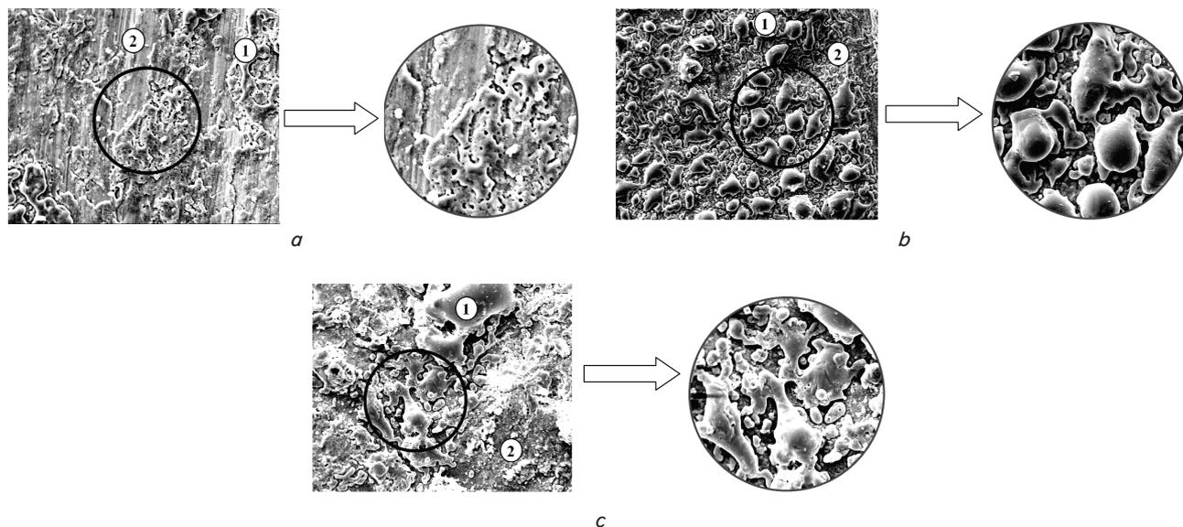
Fig. 4. Surface morphology of oxide coatings on AK12M2MgN, formed on electrolytes of following composition, mol/dm<sup>3</sup>:
