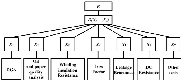
Fig. 1. The hierarchical block diagram for the technical condition assessment of power transformers
