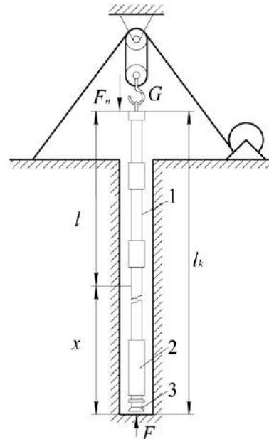
Fig. 1. Modeled scheme of drill string:
