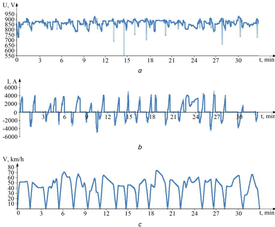
Fig. 4. Oscillograms of voltage on the current collector (a), the train current (b) and the train speed (c) during its operation between Lisova and Akadmistechko stations
