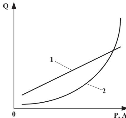
Fig. 6. Graphs of changes in the cost of storage systems depending on their power and energy intensity: dependence of  $Q = f(P)$  at  $A = \text{const}$  (1); dependence  $Q = f(A)$  at  $P = \text{const}$  (2)
