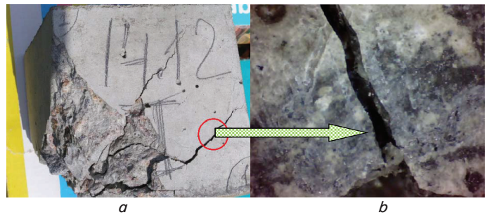
Fig. 4. Sample-cubes of concrete of the control composite after tests for a high-velocity impact: a – general view; b – microstructure
