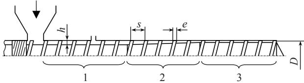
Fig. 1. Schematic of the classical three-zone single-screw extruder: 1, 2, 3 – feeding, melting and homogenization zones;  $D$ ,  $h$  and  $e$  – a diameter, a height and a width of the ridge of the screw thread,  $m$ ;  $s$  – a step of angular thread,  $m$
