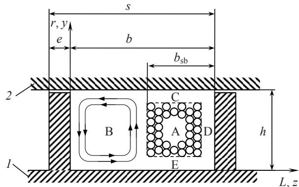
Fig. 3. The mechanism of melting of a polymer in the working channel of a single-screw extruder: 1 – a screw; 2 – a cylinder; A, B, C, D, E – areas of the working channel in the boundaries of the melting zone of the extruder;  $z, L$  – coordinates directed along the axis of the screw,  $m$ ;  $r, y$  – coordinates directed along the height of the channel of the screw,  $m$ ;  $b$  – a width of the screw channel,  $m$ ;  $b_{sb}$  – a width of a solid polymeric “solid bed”,  $m$
