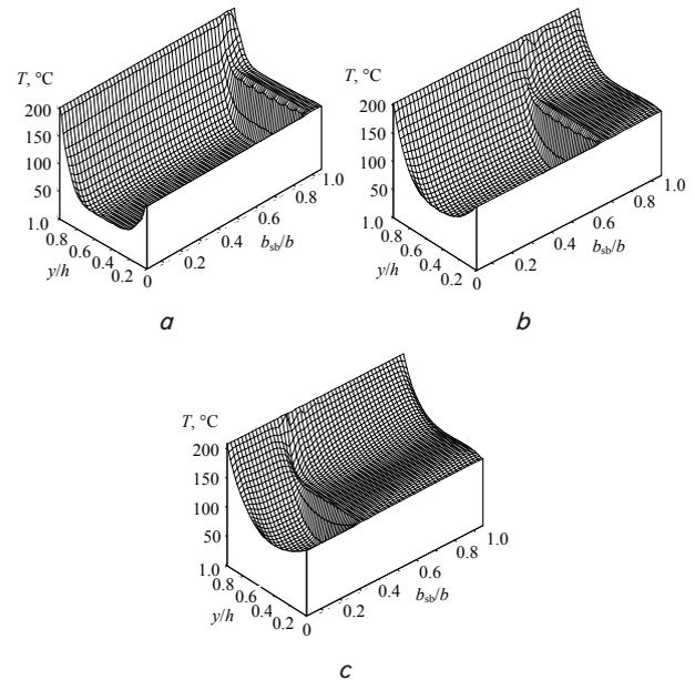
Fig. 5. Temperature fields in the screw channel at different values of the dimensionless coordinate  $L/D$ :  $a - 6.0$ ;  $b - 8.0$ ;  $c - 12.5$  ( $b_{sb}/b$  – dimensionless width of the “solid bed”;  $y/h$  – dimensionless height of the working channel)
