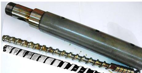
Fig. 2. Physical appearance of the screw extracted from an extruder body (light color highlights the melt solidified in the screw channel)
