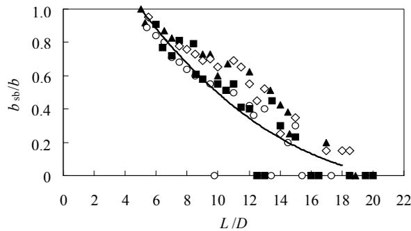
Fig. 6. Comparison of experimental data [12] with the calculation results according to the developed method (screw rotation speed 40 rpm, mass performance 32.6 kg/h; markers show the results of measurements of four series of experiments)
