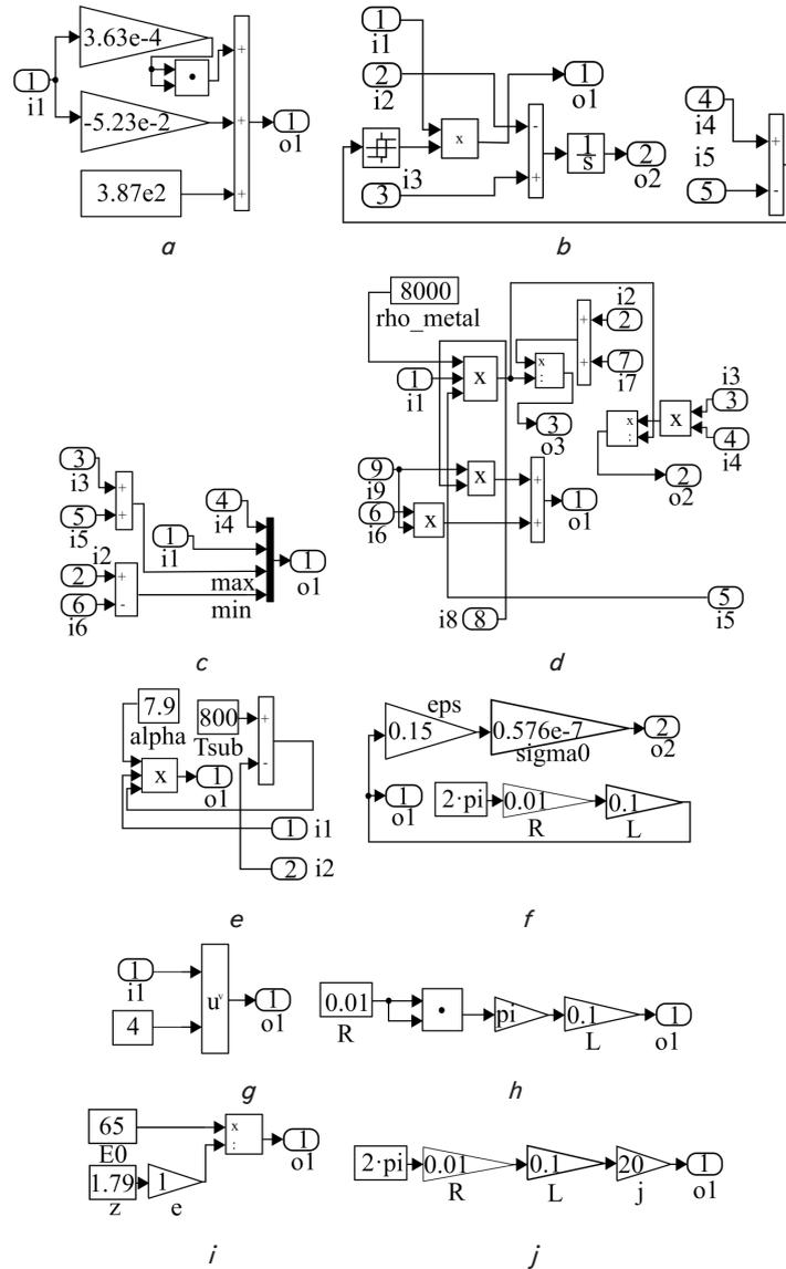
Fig. 3. Subsystems of the model (designations correspond to Fig. 2): a – HeatCup, b – Relay\_Integrator, c – Display, d – main\_eq, e – alfa\_Tsub, f – s\_and\_a1, g –  $\cdot^4$ , h –  $R^2 \cdot \pi \cdot L$ , i –  $E0 / (z \cdot e)$ , j –  $2 \cdot \pi \cdot R \cdot j$
