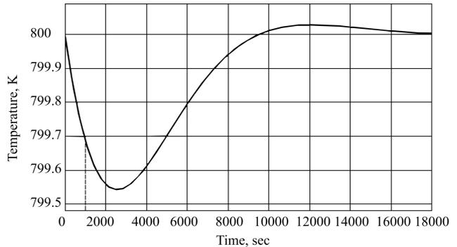
Fig. 8. Transient process of change in the tool temperature under the action of maximum disturbance
