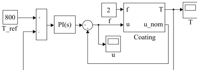
Fig. 6. Simulation model of the temperature stabilization system at the stage of applying a coating on the tool
