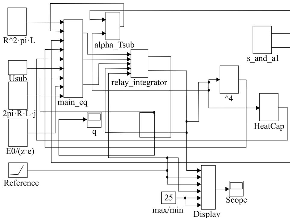
Fig. 2. Simulation model of the ionic cleaning control system
