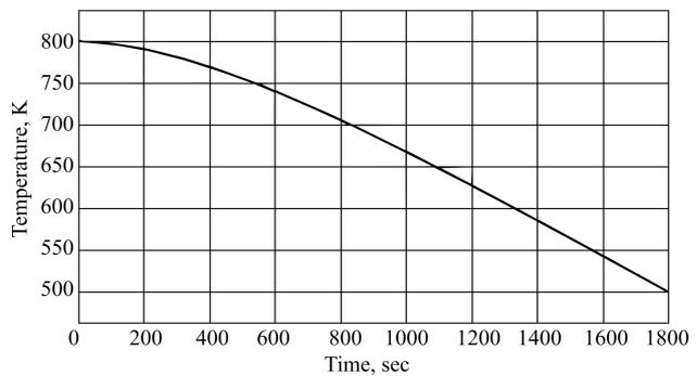
Fig. 16. Process of the programmed change in the tool temperature
