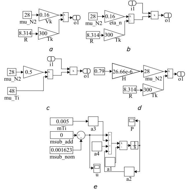
Fig. 11. Subsystems of the model for a pressure control system: a – subsystem a1; b – subsystem a2; c – subsystem a3; d – subsystem a4; e – subsystem Pressure
