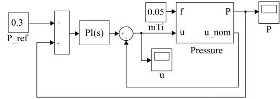
Fig. 10. Simulation model of the pressure control system
