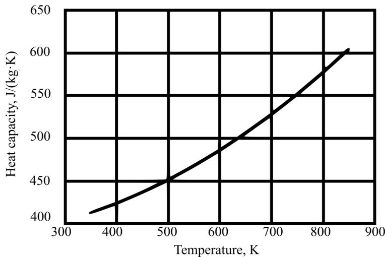
Fig. 1. Chart of change in the heat capacity of steel
