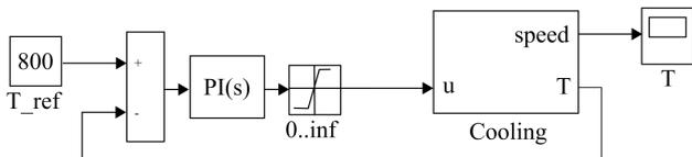
Fig. 14. Simulation model of the cooling control system
