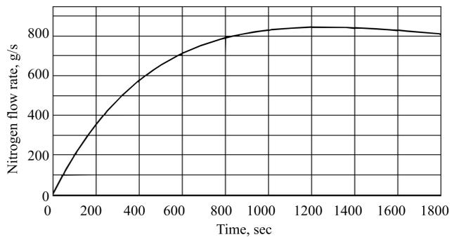
Fig. 17. Transient process of change in control at the stage of cooling
