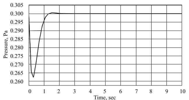
Fig. 12. Transient process of change in the nitrogen pressure under a disturbance by increasing mTi
