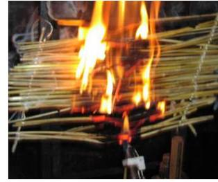
Fig. 4. Results of determining the flammability of a reed sample under the action of a burner
