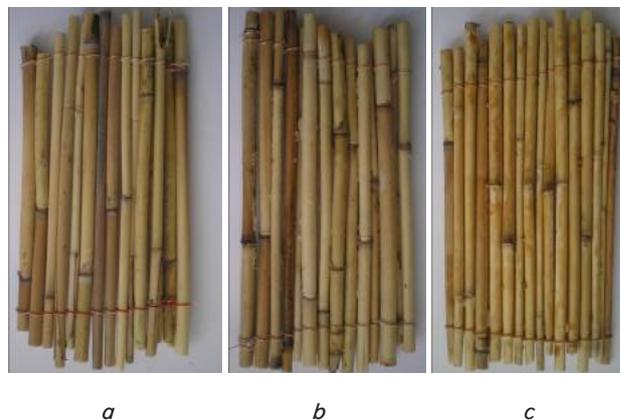
Fig. 1. Model samples of fire-retardant reed: *a* – raw, *b* – treated with a fire-retardant impregnating composition; *c* – treated with a flame-retardant coating
