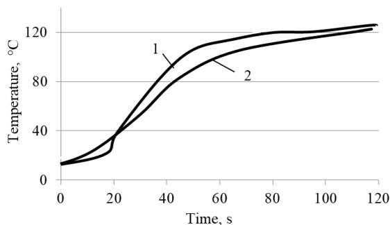
Fig. 7. Dynamics of temperature gain by the inner wall during tests of fire-retardant reed: 1 – treated with an impregnating composition, 2 – treated with a swelling coating
