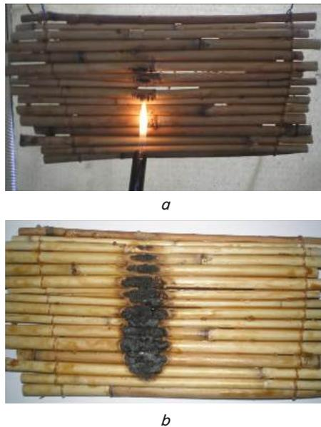
Fig. 6. Test results of reed protected from fire by a swelling coating: *a* – effect of flame of the burner on reed; *b* – formation of a thermally-insulating coke layer at the surface of a combustible substance
