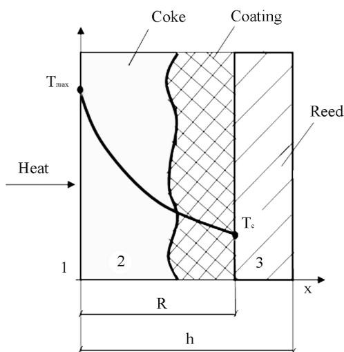
Fig. 3. Schematic of the swelling process of a flame-retardant coating: 1 – outer environment; 2 – a layer of coked foam; 3 – source material (reed)
