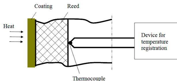
Fig. 2. Device for studying the thermal conductivity of reed
