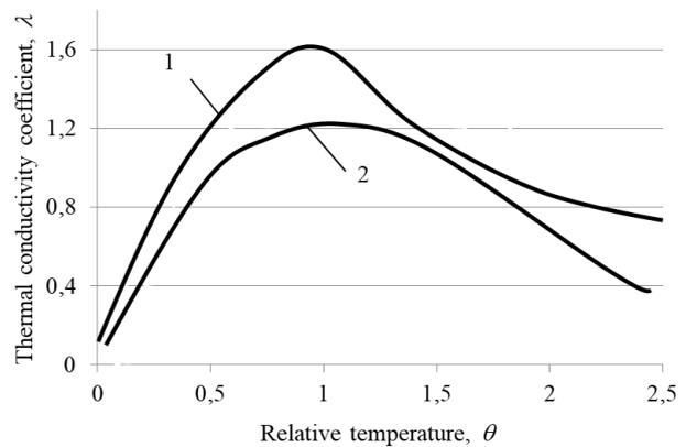
Fig. 8. Thermal conductivity coefficient dependence on the temperature of heating environment: 1 – a fire-retardant impregnation agent, 2 – a coating
