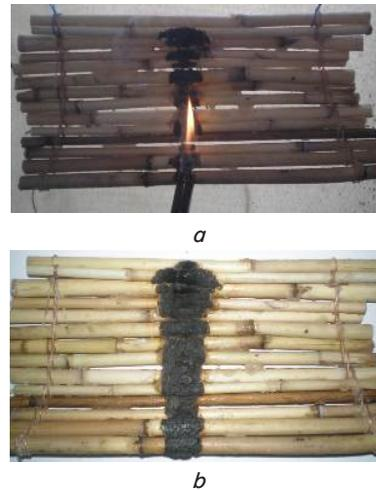
Fig. 5. Test results of reed protected from fire by an impregnating agent: *a* – effect of flame of the burner on reed; *b* – formation of a coke layer at the surface of a combustible substance
