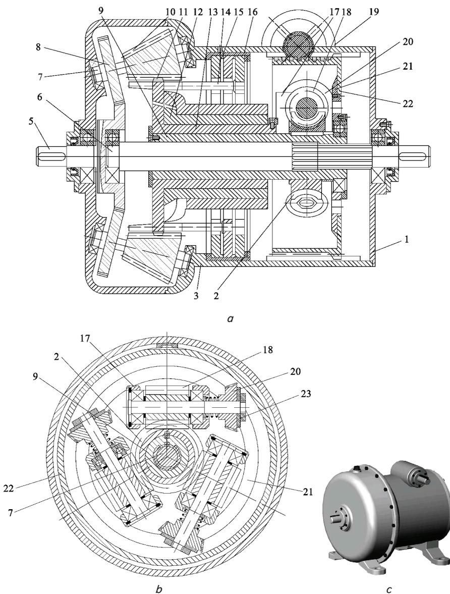
Fig. 2. Design of the CVT: a – longitudinal cross-section; b – transverse cross-section; c – solid model
