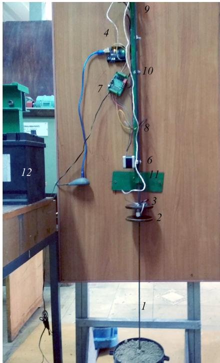
Fig. 3. Appearance of the information-measuring system of soil penetration (designation according to Fig. 3)
