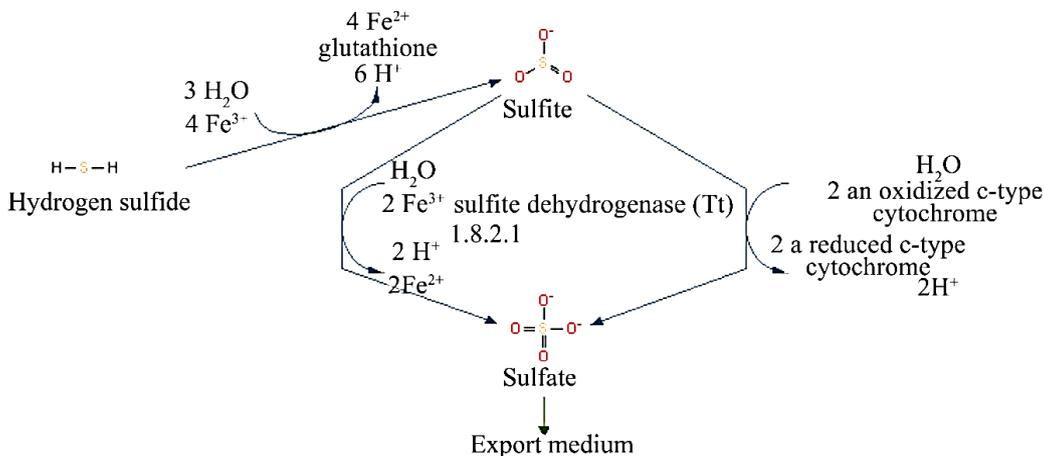
Fig. 8. Schematic of sulfide-oxidation of metabolic process of *Acidithiobacillus ferrooxidans*
