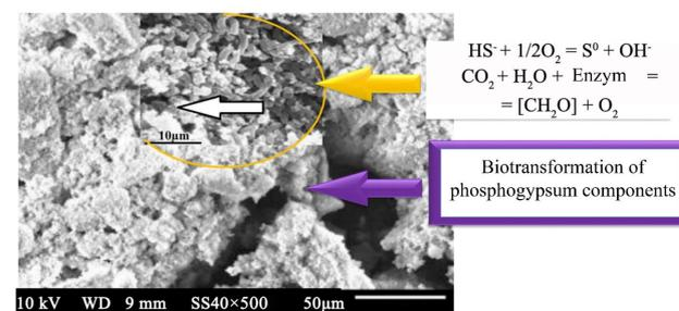
Fig. 4. Raster microscopy of biotransformations of phosphogypsum granules in the process of oxidation of hydrogen sulfide with thiobacteria. The arrows of different colors show: white – clusters of the formed biosulfur (GS. 10 μm); yellow – bioactive layer in a crack of modified phosphogypsum granules (GS 10 μm); purple – the zone of a crack of a biotransformed granules (GS 50 μm)
