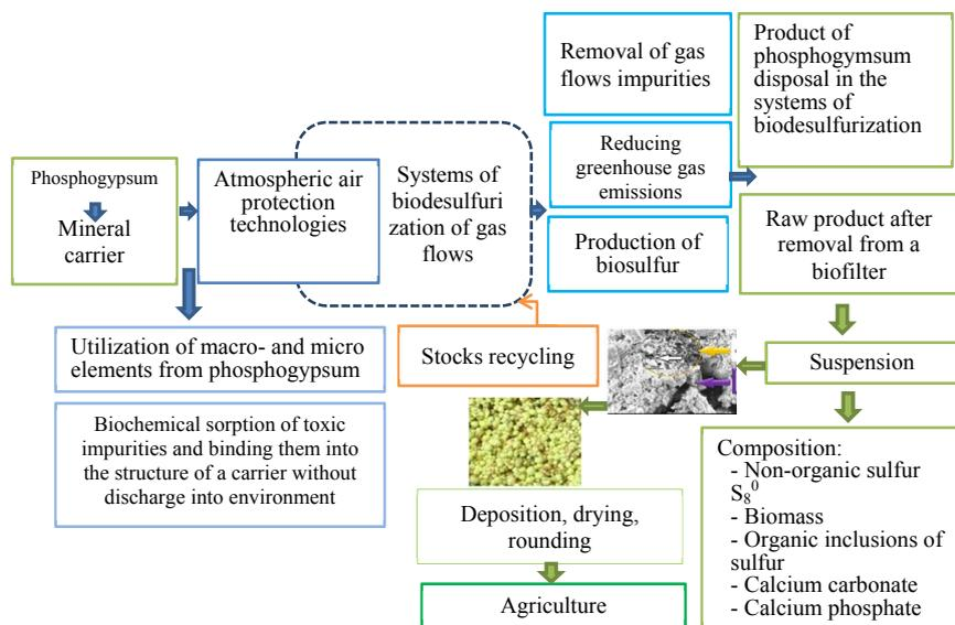
Fig. 11. General block diagram of integrated environmentally safe process of phosphogypsum disposal with obtaining biosulfur as the disposal product
