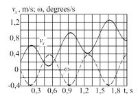
Fig. 7. The law of change in the trolley motion speed projection across the span  $v_x$  and in the angular velocity  $\omega$  at the initial stage of motion with an initial speed of  $v_x$ =0.2 m/s
