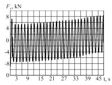
Fig. 11. The law of change in the tangent dynamic load
