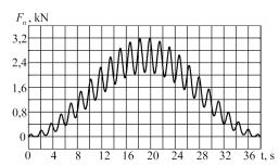
Fig. 12. Change in the normal dynamic loading (break of a traction winch rope)
