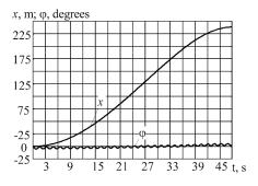
Fig. 3. The law of change in the displacement of trolley x across the span and in angle of the load deviation from the vertical  $\phi$  over time t
