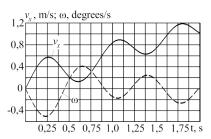
Fig. 8. The law of change in the speed of trolley displacement across the span  $v_x$  and in the angular velocity  $\omega$  at the initial stage of motion at a short release of the carrying rope tension  $H_x$ =7.5·10<sup>5</sup> N
