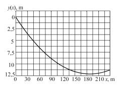
Fig. 9. Calculated trajectory of the trolley motion y(x)
