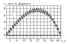
Fig. 4. The law of change in the trolley displacement speed vx across the span and in the load angular velocity  $\omega$  over time t
