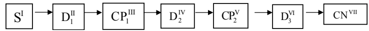
Fig. 4. The scheme of delivery of cargo in a container from A to B by sea freight and by maritime transport I, II,...,VII – the numbers of delivery route stages; S – a supplier; CN – a consumer; D 1 – delivery of cargo by motor transport from the Customs Office in the country of shipment to the port in a country of shipment, D 2 – delivery of goods by sea freight, D 3 – delivery of goods by motor transport from the port of arrival to the Customs Office of destination; CP 1 – servicing at the port of shipment, CP 2 – servicing at the port of destination
