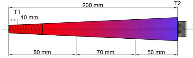
Fig. 3. Thermocouple positions
