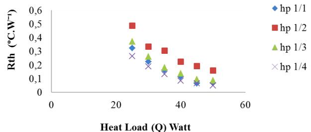
Fig. 8. Thermal resistance by heat load
