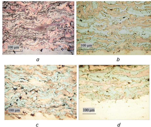
Fig. 3. Microstructure of electric-arc pseudoalloy coatings: a – Cu-NiCr; b – Cu-Mo; c – Cu-Ti; d – Cu-FCW(FeB)
