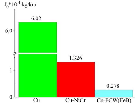
Fig. 5. Results of tests of pseudoalloy coatings for wear at the temperature of ( $J_0$ ) as compared to pure copper
