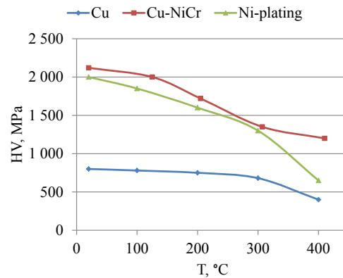
Fig. 6. Dependence of the hot hardness (HV) of pure copper, Ni-plating and pseudoalloy coating of Cu-NiCr on the temperature (T)
