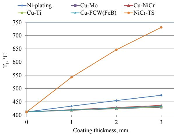
Fig. 2. Value of the temperature of the outer wall of the mold ( $T_1$ ) depending on the thickness and type of coating
