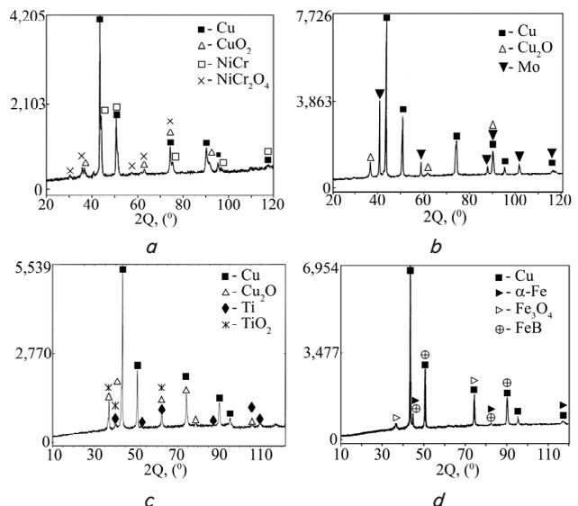
Fig. 4. X-ray patterns of electric-arc pseudoalloy coatings: a – Cu-NiCr, b – Cu-Mo, c – Cu-Ti, d – Cu-FCW(FeB)
