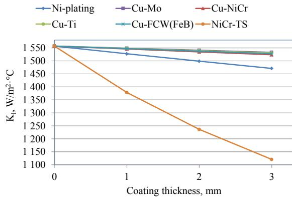
Fig. 1. Dependence of the heat transfer coefficient ( $K_p$ ) in the upper part of the mold on the thickness and type of coating
