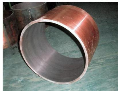
Fig. 7. Fragment of the CCM mold liner with the inner Cu-NiCr coating after machining
